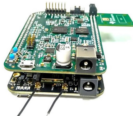
図 26. DSP Board Sitting on top of BeagleBone™ Black Wireless With DC Jacks Aligned
