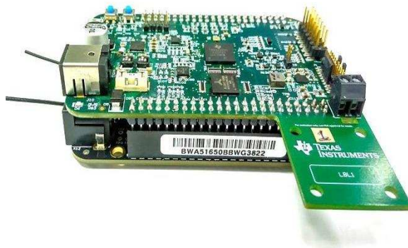
図 25. DSP Board Sitting on top of BeagleBone™ Black Wireless
