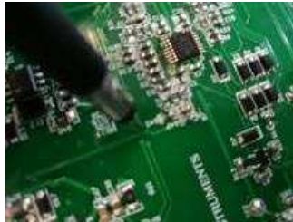
38. Floating Probe Close to Input Path of the Amplifier
