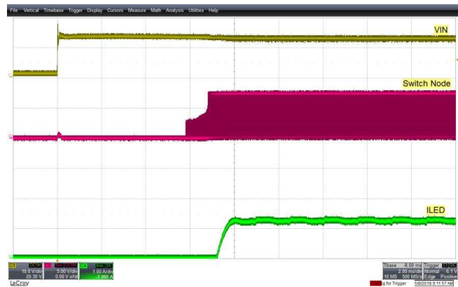
Figure 10 . High Beam/Low Beam Mode Steady State Switching—CH2: Switch Node (Q3 Drain) Voltage and CH4: LED Current for Output power of 55 W
