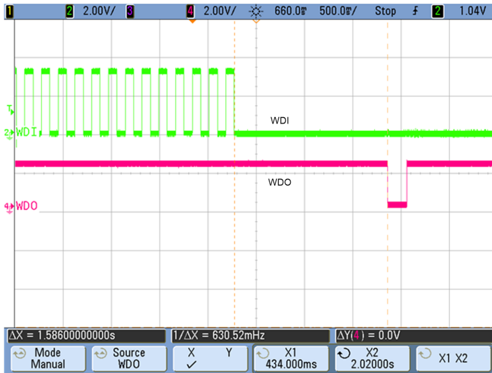
Figure 26. WDT Configuration 2: Timeout of 1600 ms
