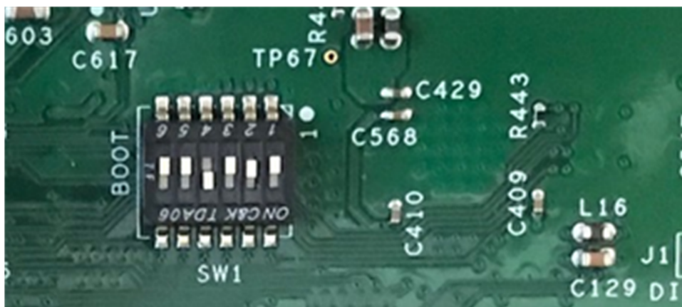
Figure 9. Boot Mode Switch SW1 Settings
