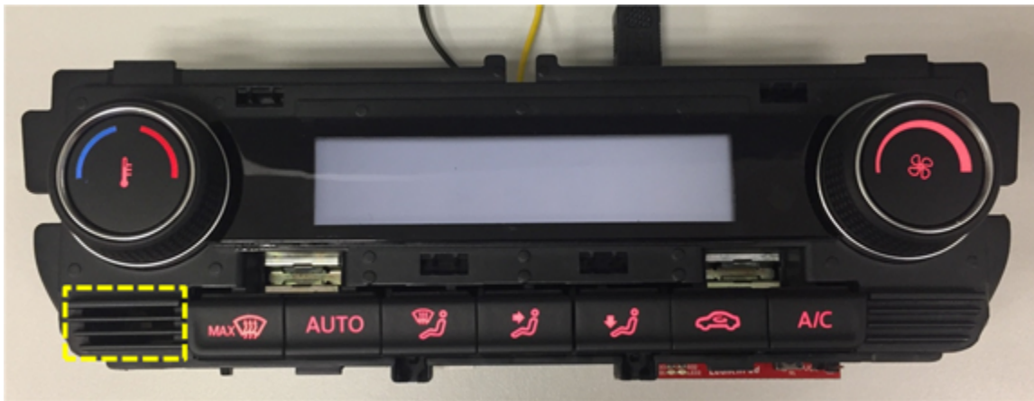
図 12. HVAC HMI Housing
