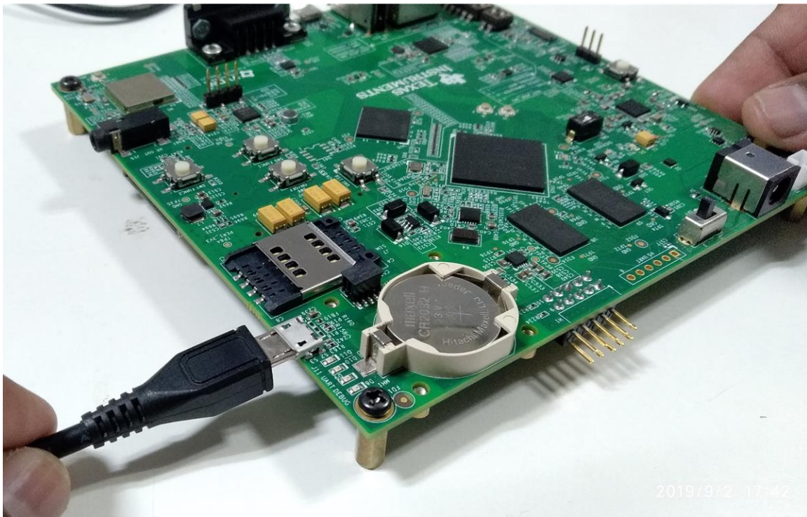
図 27. Inserting micro-B Cable Into J11
