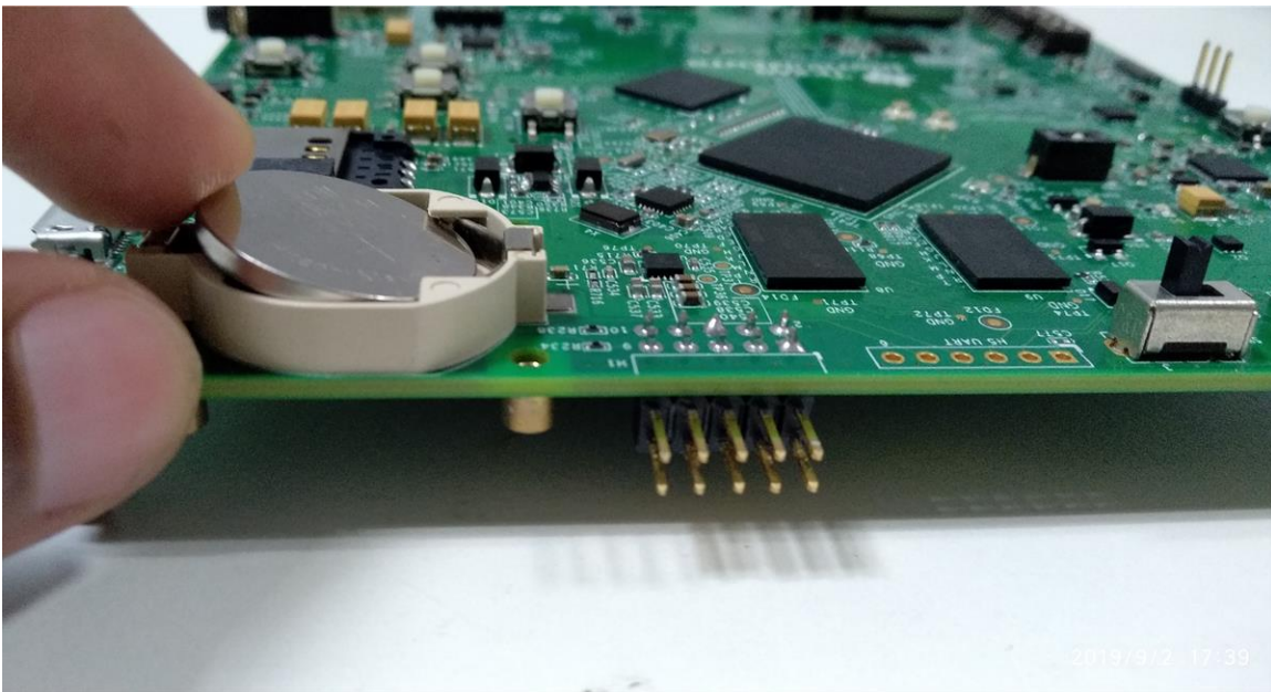
図 25. Inserting Coin Cell Battery Into BH1
