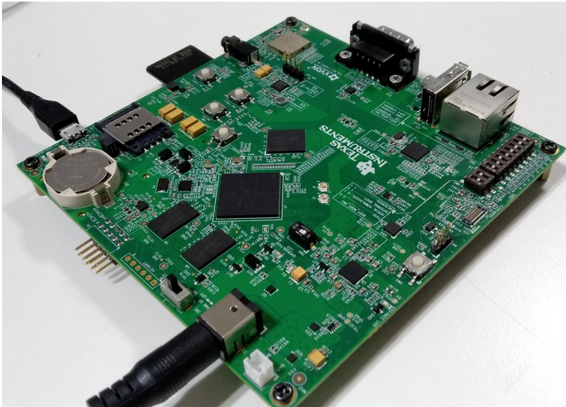
図 29. Board Connections for BOOT From SD Card With Debug Over USB
