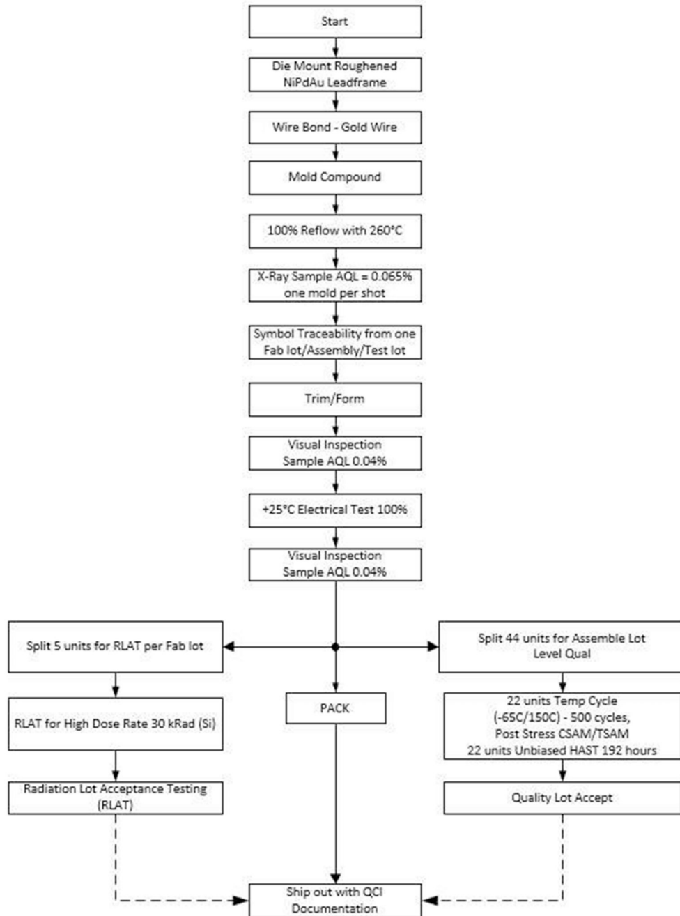
Figure 2-1. ADC168M102R-SEP Space-Enhanced Plastic Production Flow Chart
