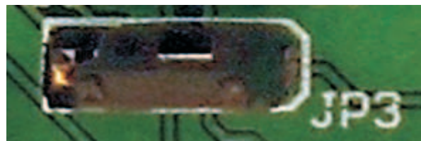
Figure 1. Reference Selection Jumper JP3
