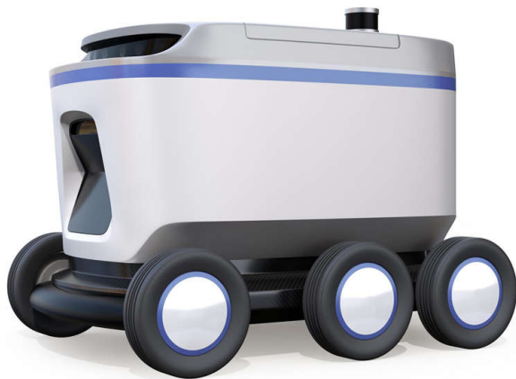
Figure 2. Autonomous Mobile Robots (AMR) Featuring a Mechanically Scanning LiDAR Module on the Top
