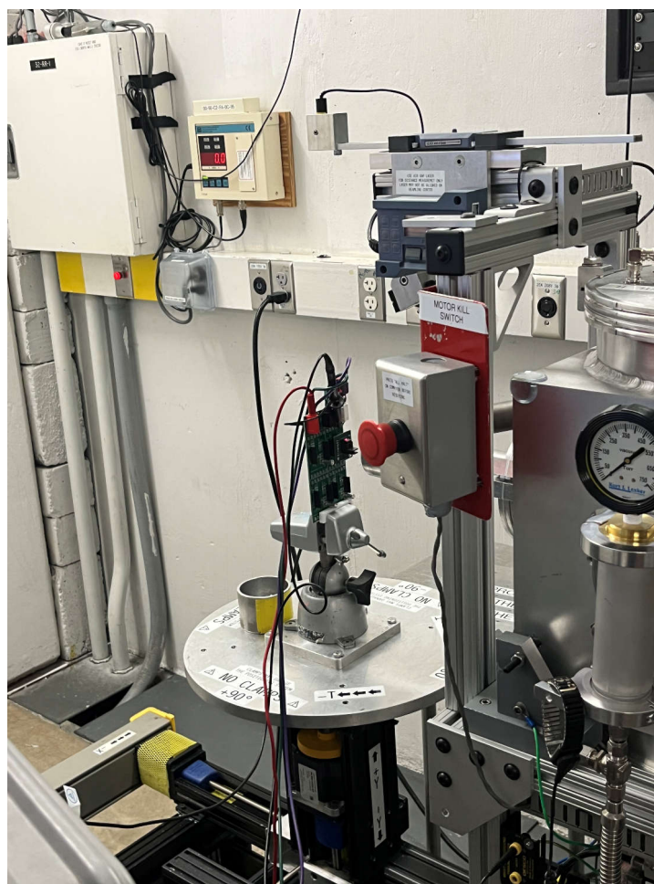
Figure 4-1. Photograph of the OPA4H199-SP EVM in Front of the Heavy-Ion Beam Exit Port at the Texas A&M Cyclotron
