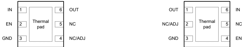
Figure 4-3. Pin Diagram (DRV Package (Fixed/ADJ), 6-Pin WSO N , Top View) Figure 4-4. Pin Diagram (DRV Package, A-version (Fixed/ADJ), 6-Pin WSO N , Top View)
