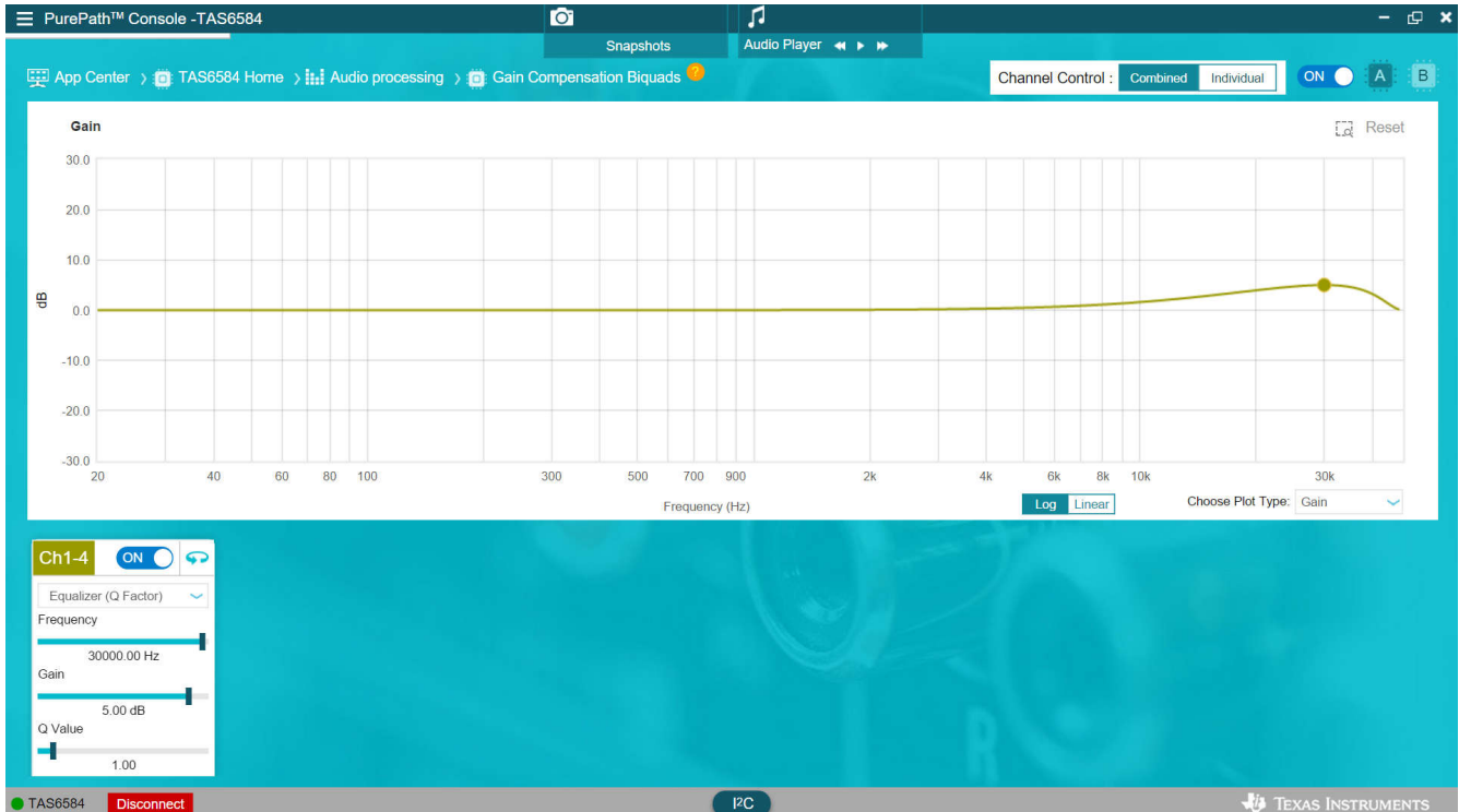
Figure A-2. TAS6584-Q1 GUI Gain Compensation Biquads Page - 2Ω
