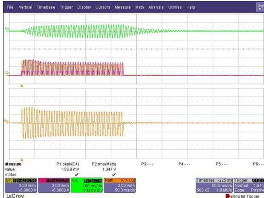
Figure 8. Strong Buzz Waveform for LRA in Auto-Resonance Mode
