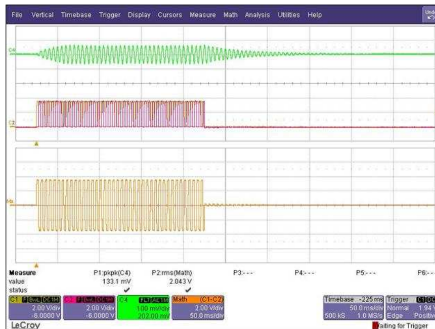
Figure 9. Strong Buzz Waveform for LRA in Open-Loop Mode
