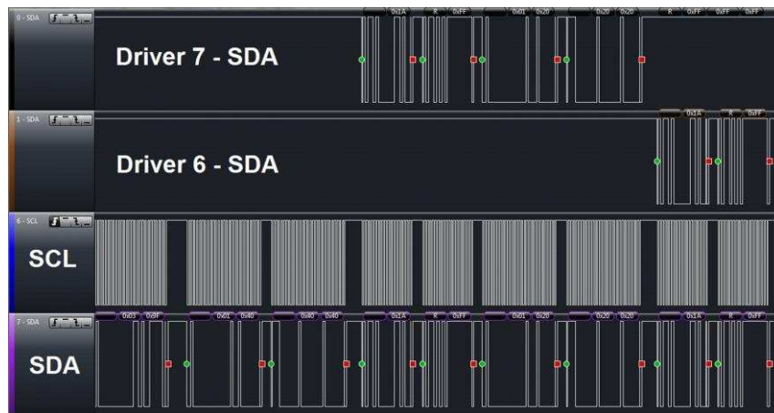
Figure 10. TCA9548A Logic Analyzer Operation
