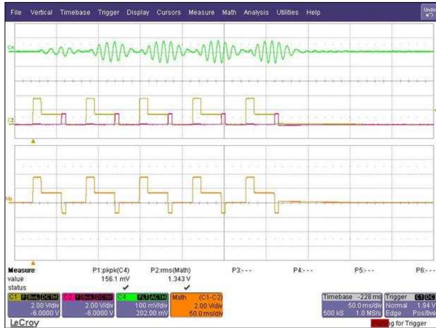
Figure 7. Pulsing Strong waveform for ERM in Open-Loop Mode
