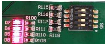
Figure 64. CPLD Switches and LEDs
