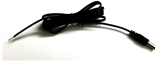
Figure 2. Provided Power Cable for J1 Connector
