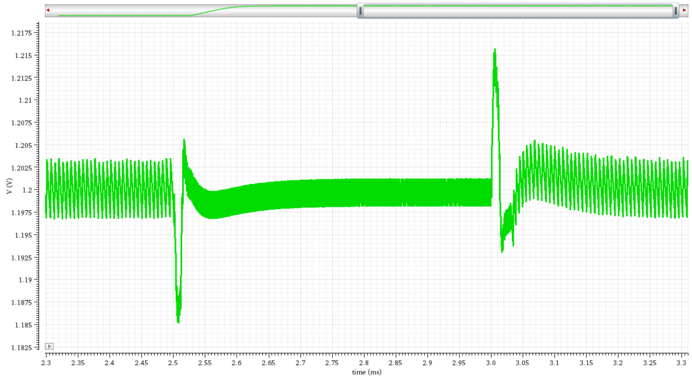
Figure 2-9. Cadence Load Transient Simulation Waveform
