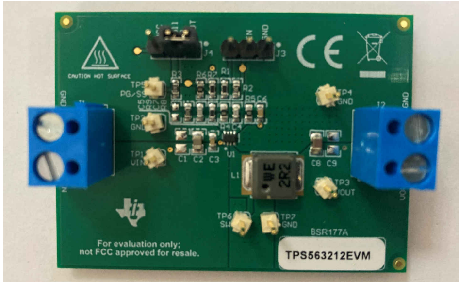
Figure 5-4. TPS563212EVM Board (Top View)
