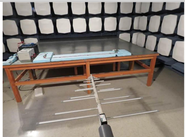
Figure 7. Test Setup for Radiated Emission Measurement: 200-MHz to 1000-MHz (Horizontal Log Antenna)
