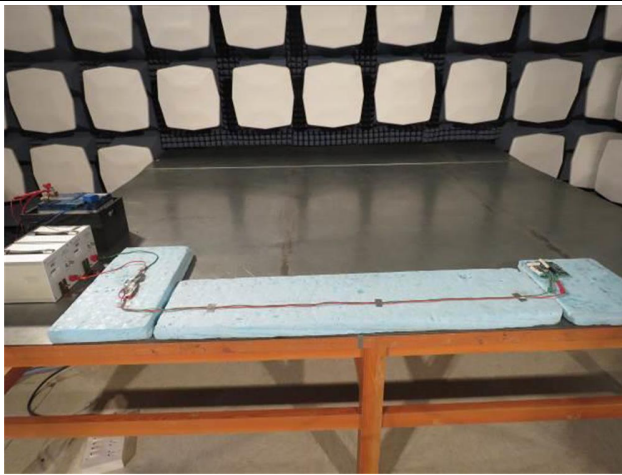
Figure 2. Test Setup for Conducted Emission Measurement
