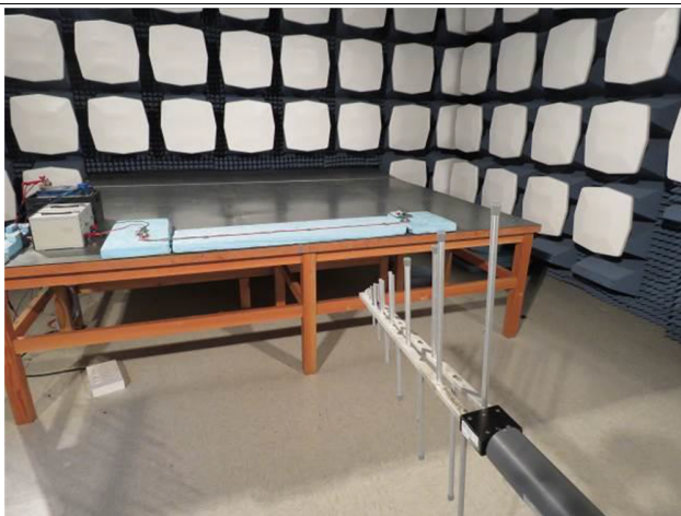
Figure 6. Test Setup for Radiated Emission Measurement: 200-MHz to 1000-MHz (Vertical Log Antenna)
