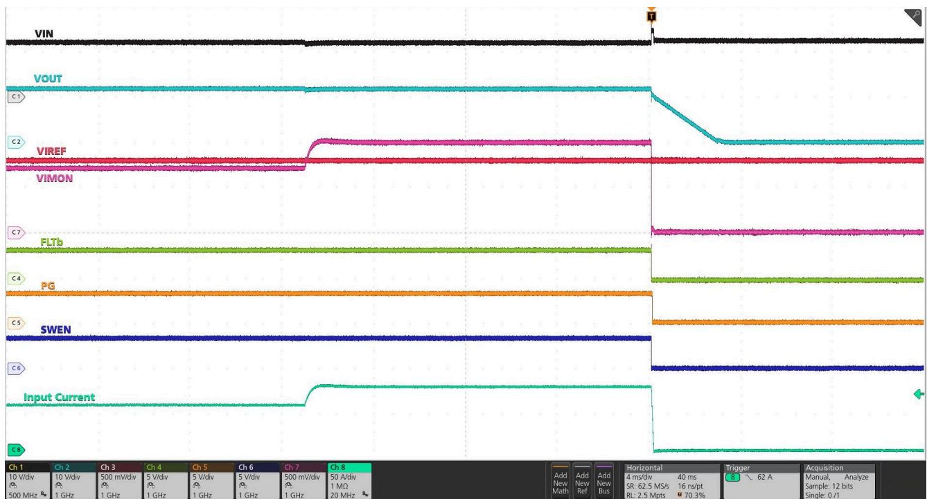
Figure 4-3. Over-current Protection in TPS25990 eFuse
