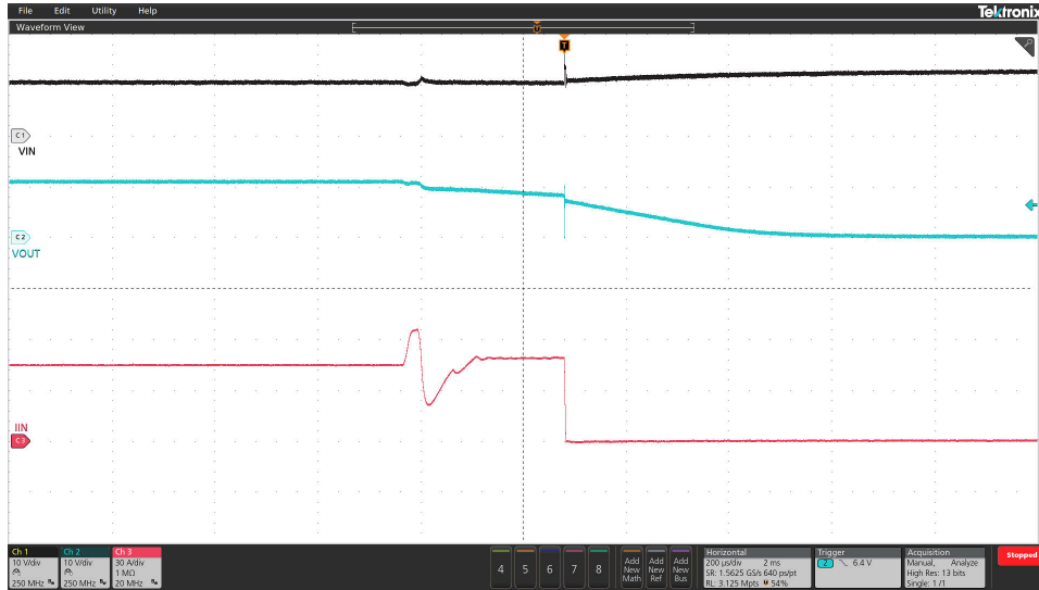
Figure 2-1. Over-Current Response of the Conventional eFuse-1
