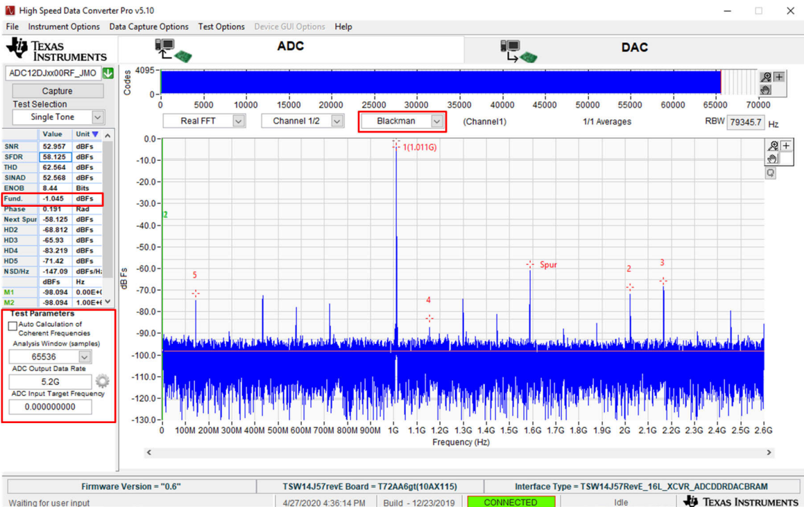
Figure 4-1. Example FFT Plot of the ADC12DJ5200RF Using Noncoherent Sampling
