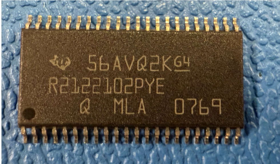
Figure 1-1. TPS7H4011-SP QMLP Device Used in Exposure (Front)
