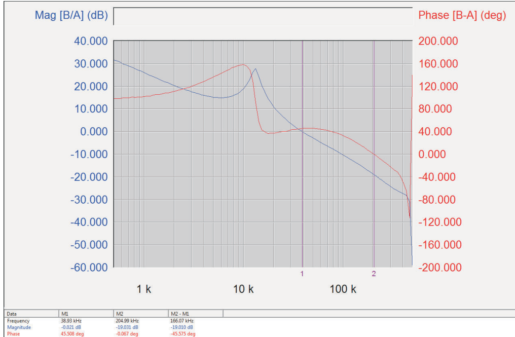
Figure 9-11. Loop Gain ( V_{IN} = 12\text{ V} , V_{OUT} = 1.0\text{ V} , I_{OUT} = 15\text{ A} , Bandwidth: 39 kHz, Phase Margin: 46°)
