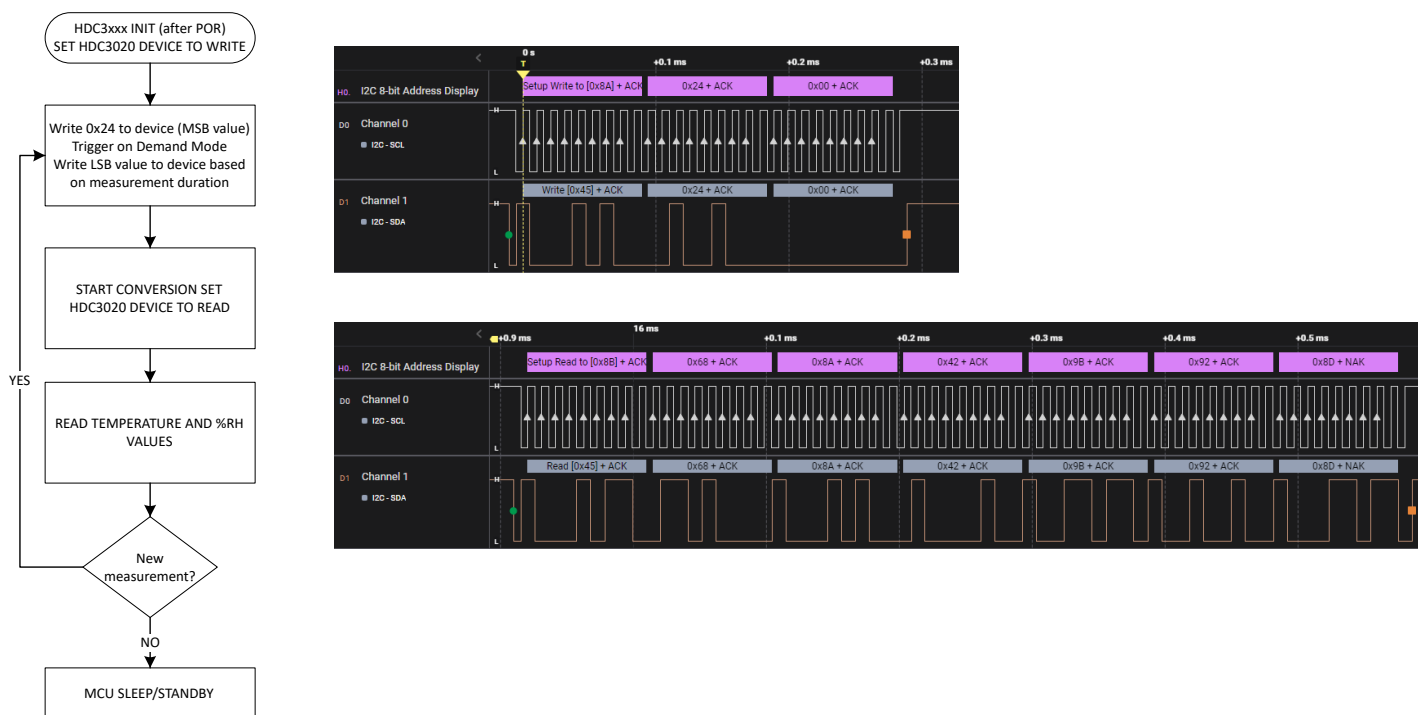
Figure 3-1. Flowchart for Trigger-On Demand Mode
