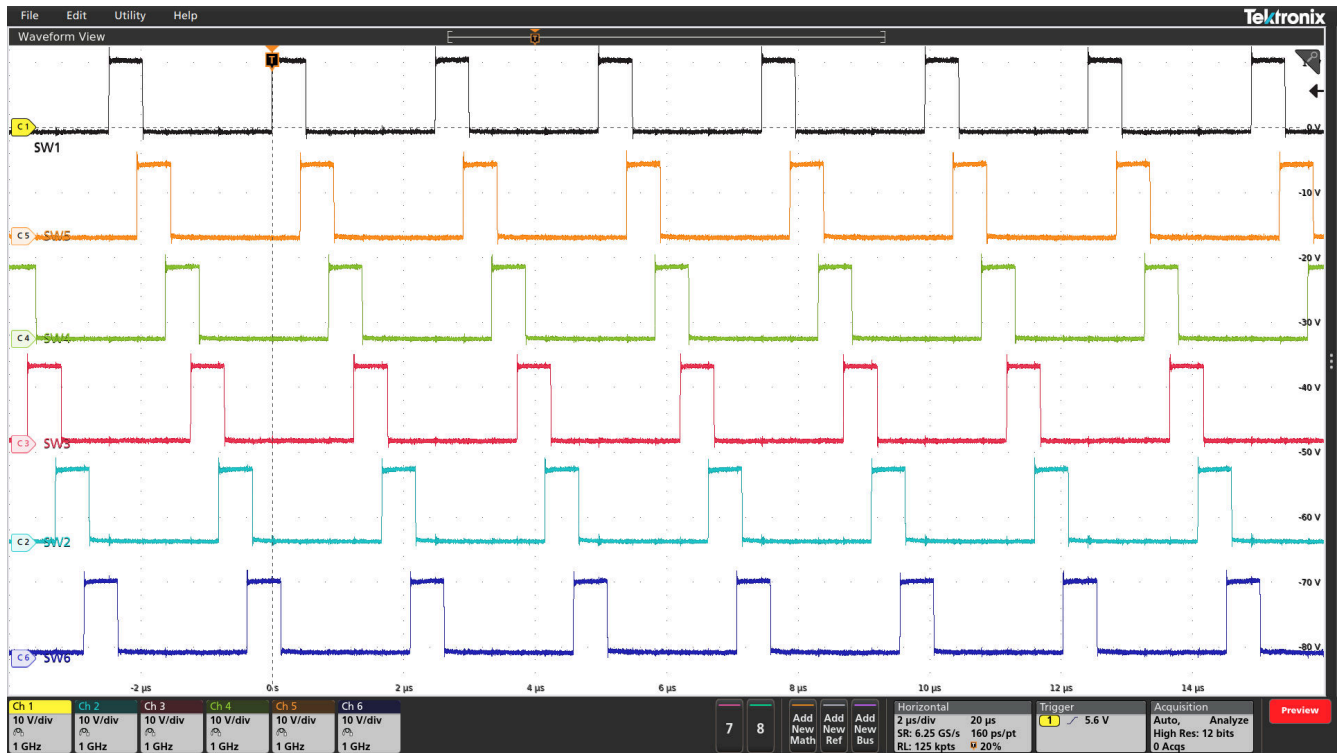
Figure 5-7. SW Node Voltage, V_{IN} = 12\text{ V} , V_{OUT} = 3.3\text{ V} , I_{OUT} = 2\text{ A} , FPWM mode
