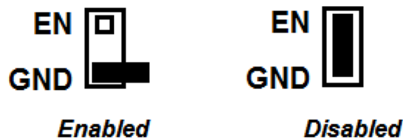
Figure 2. Enable Jumper Setting
