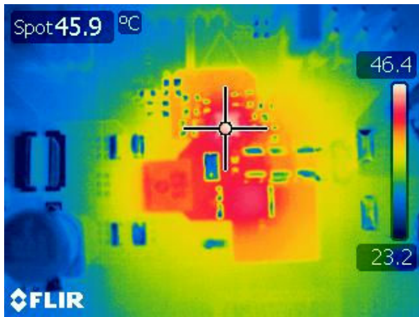
Figure 5-5. Thermal Image V_{IN} = 6\text{ V} I_{OUT} = 1.6\text{ A} , V_{BIAS} = V_{IN} , no Forced Air Cooling
