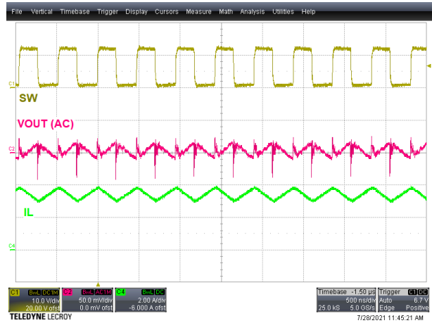
Figure 5-8. Steady State, V_{IN} = 6\text{ V} , I_{OUT} = 1.6\text{ A}
