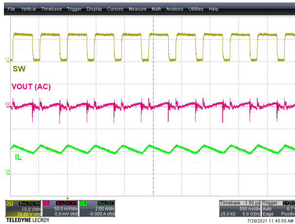
Figure 5-9. Steady State, V_{IN} = 9\text{ V} , I_{OUT} = 1.6\text{ A}
