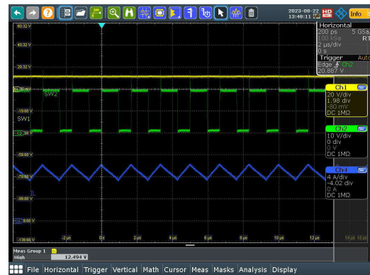
Figure 3-11. SW1, SW2, I_L ( V_{IN} = 12V , I_{OUT} = 5.0A )
