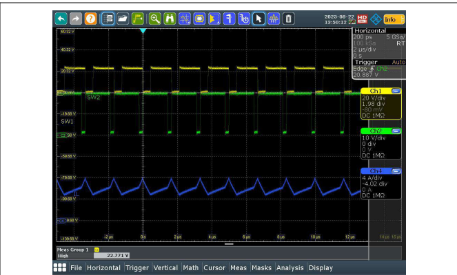
Figure 3-15. SW1, SW2, I_L ( V_{IN} = 24V , I_{OUT} = 5.0A )
