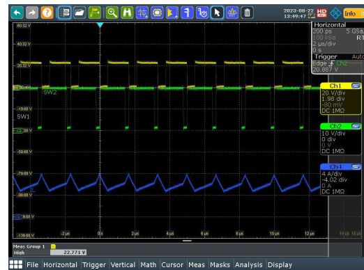
Figure 3-13. SW1, SW2, I_L ( V_{IN} = 16V , I_{OUT} = 5.0A )
