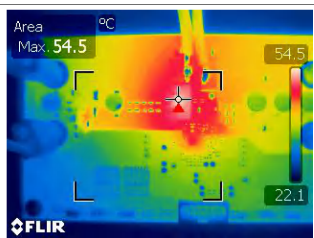
Figure 3-3. Thermal Image: V_{IN} = 16.0V , I_{OUT} = 5.0A , No Forced Air Cooling
