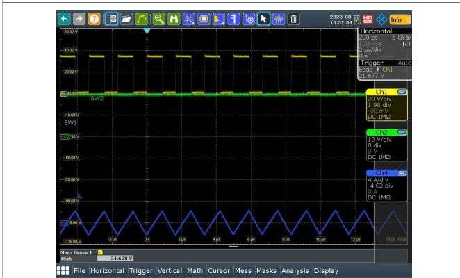
Figure 3-16. SW1, SW2, I_L ( V_{IN} = 36V , I_{OUT} = 0A )
