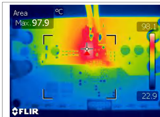
Figure 3-2. Thermal Image: V_{IN} = 9.0V , I_{OUT} = 5.0A , No Forced Air Cooling
