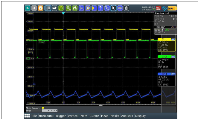
Figure 3-14. SW1, SW2, I_L ( V_{IN} = 24V , I_{OUT} = 0A )
