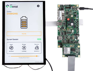
Figure 1. EV Charging Station HMI Subsystem
