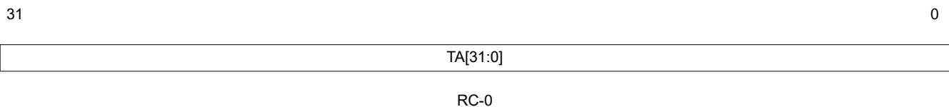
Figure 16-13. Transmission-Acknowledge Register (CANTA)
