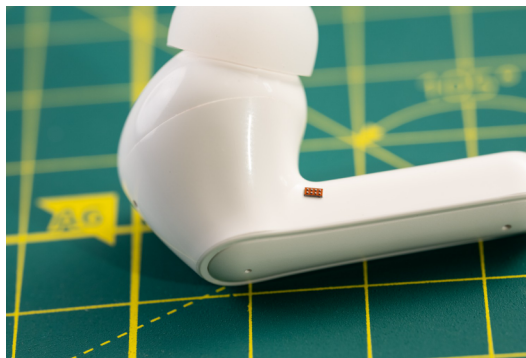
Figure 5. Size comparison between an MSPM0C1104 and a wireless earbud
