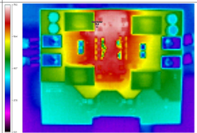
Figure 7. Rear Side: V_{IN} = 12\text{ V} , I_{OUT} = 84\text{ A}
