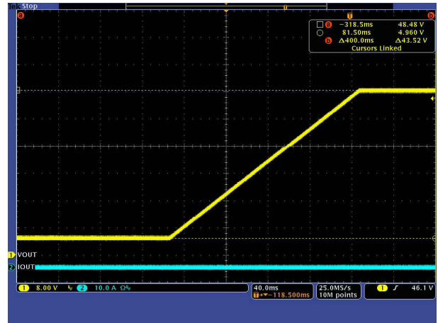
V OUT = 48 V, Prebias voltage = 5 V, no-load CH1: V OUT , CH2: I OUT
