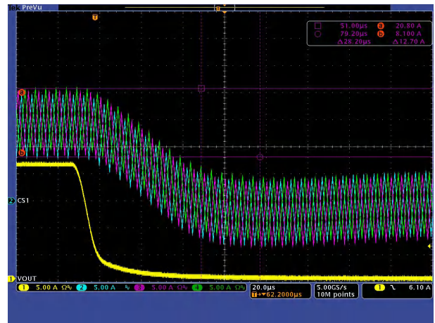
CH1: V OUT , CH2: I OUT , CH3: I Phase1 , CH4: I Phase2 Figure 3-34. V IN = 48 V, V OUT = 48 V, I OUT = 0 A to 14 A to 0 A
