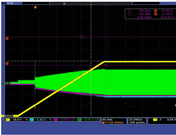
CH1: V OUT , CH2: I PHASE1 , CH3: I PHASE2 , CH4: I PHASE3 Figure 3-29. V IN = 48 V, V OUT = 48 V, I OUT = 0 A Start-Up
