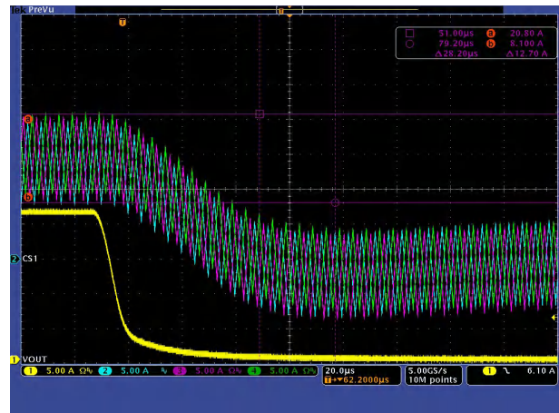
CH1: I OUT , CH2: I PHASE1 , CH3: I PHASE2 , CH4: I PHASE3 Figure 3-28. V IN = 48 V, V OUT = 48 V, I OUT = 0 A to 21 A to 0 A
