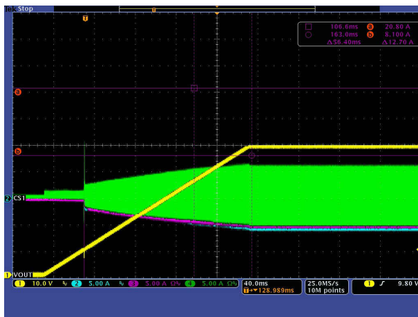
CH1: V OUT , CH2: I OUT , CH3: I Phase1 , CH4: I Phase2 Figure 3-35. V IN = 48 V, V OUT = 48 V, I OUT = 0 A, Start-up
