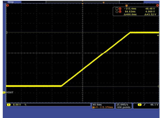
Figure 3-2. V OUT = 48 V, Prebias Voltage = 5 V, No Load CH1: V OUT
