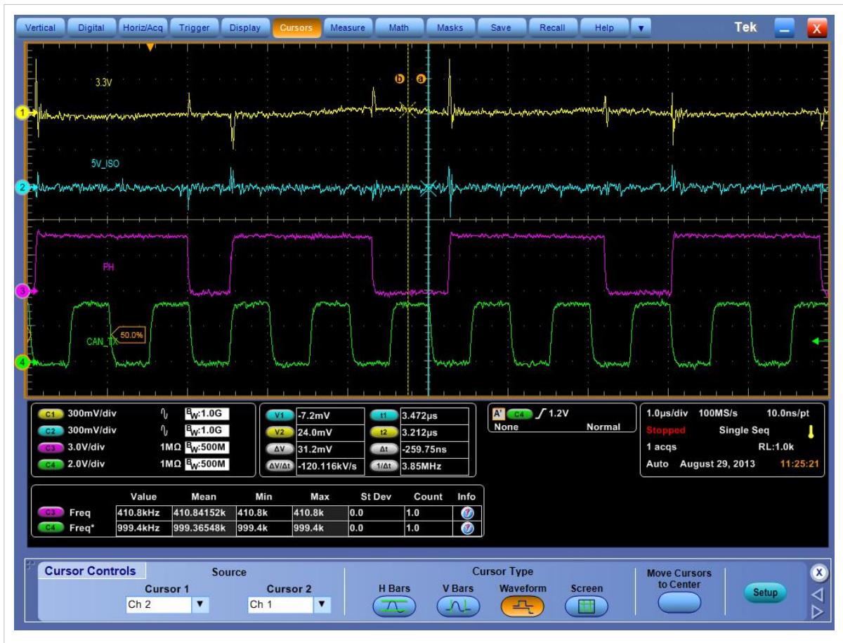
Figure 11: Output Ripple and PH node with EN enabled, Profibus (12 Mbps), CAN (1 Mbps, 50% duty cycle)
