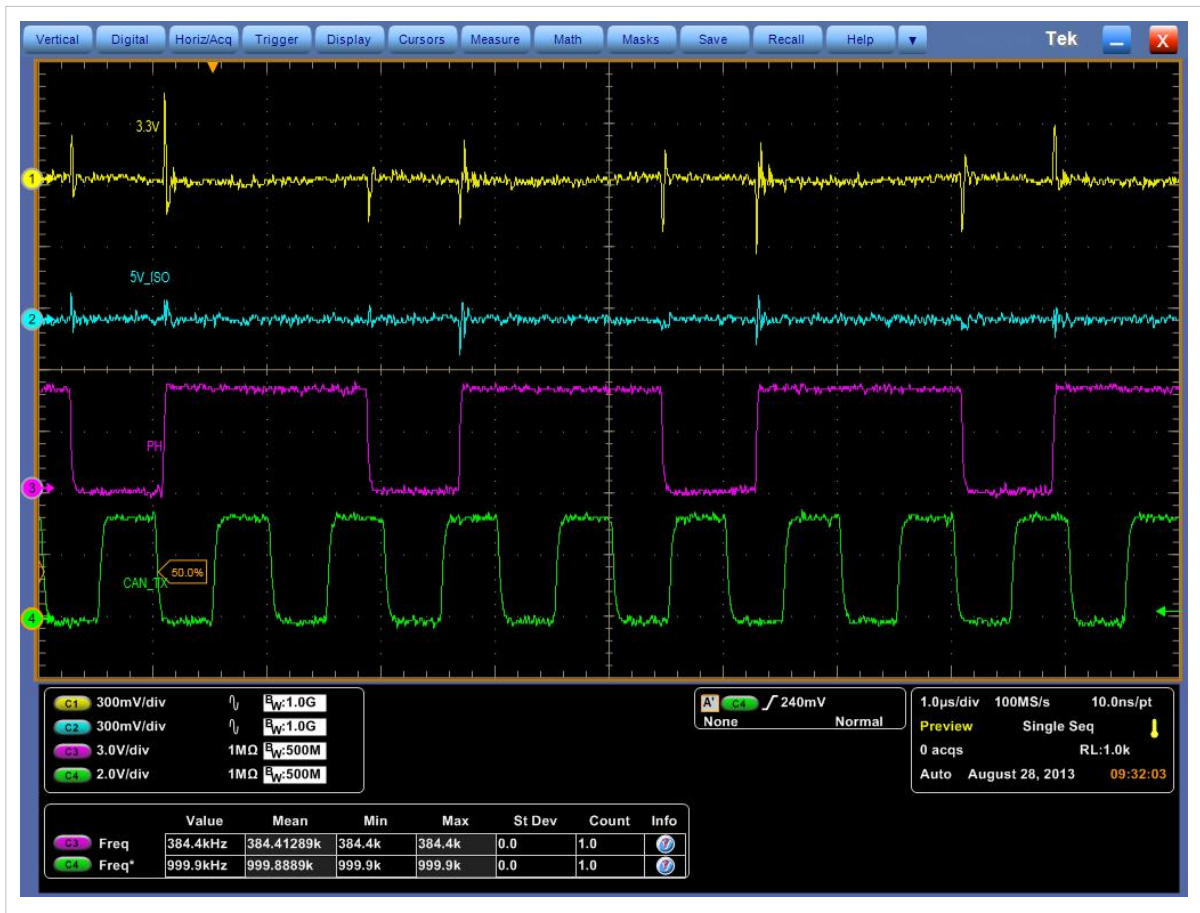
Figure 7: Output Ripple and PH node with EN enabled, CAN (1 Mbps, 50% duty cycle)
