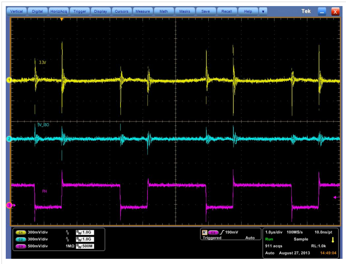
Figure 6: Output Ripple and PH node with EN enabled, no data
