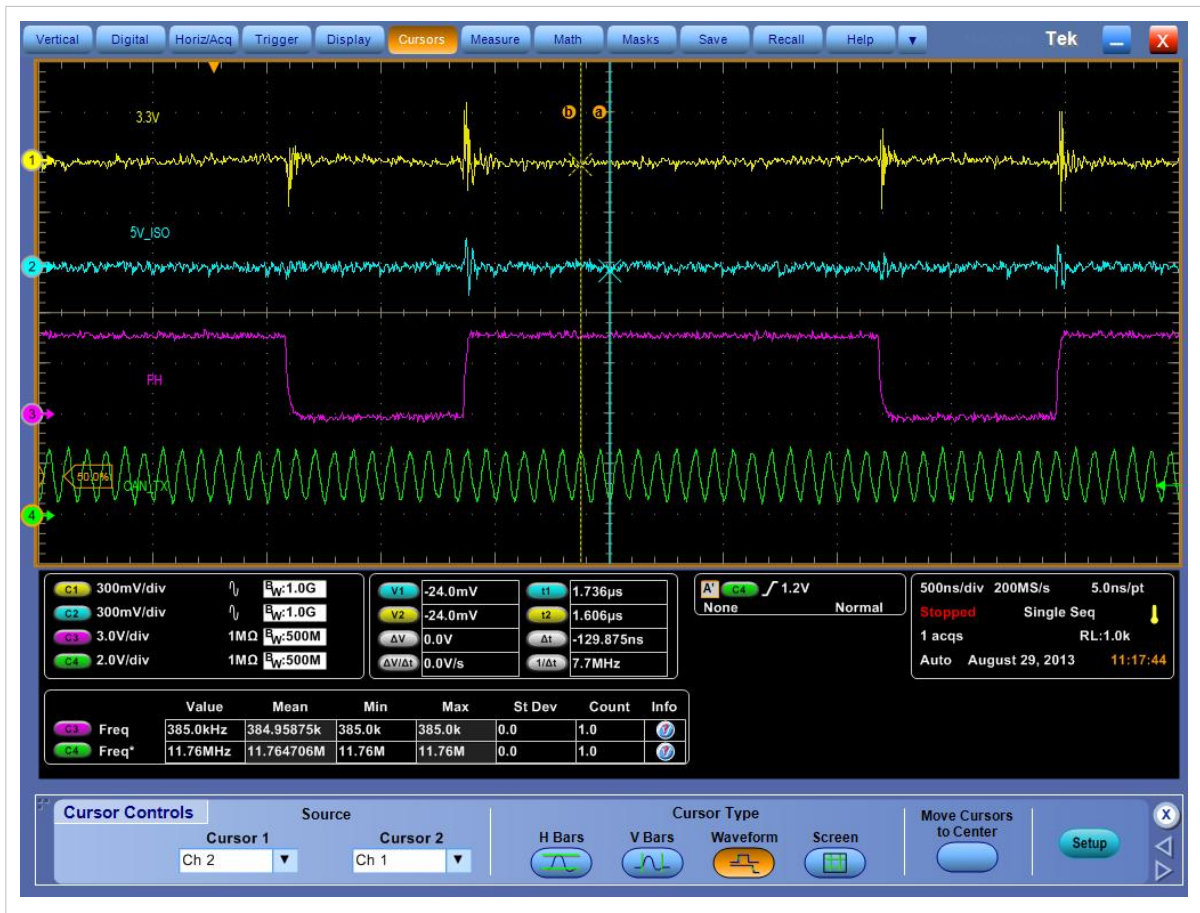
Figure 10: Output Ripple and PH node with EN enabled, Profibus (12 Mbps)
