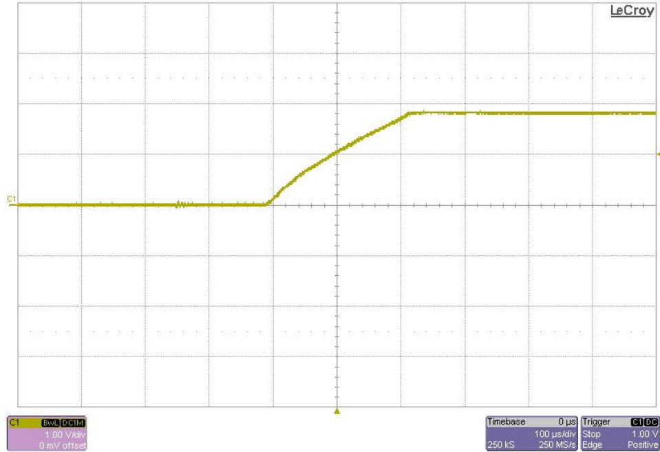
Figure 20. TLV62065EVM-719 Start-up into 2Ω Load (VIN = 5V, C1 = VOUT)
