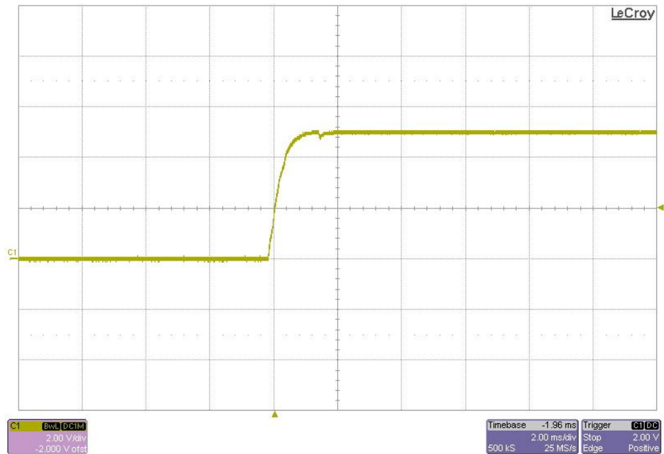
Figure 5. TPS65320EVM Start-up into 2Ω Load (VIN = 12V, C1 = BUCK_VOUT)
