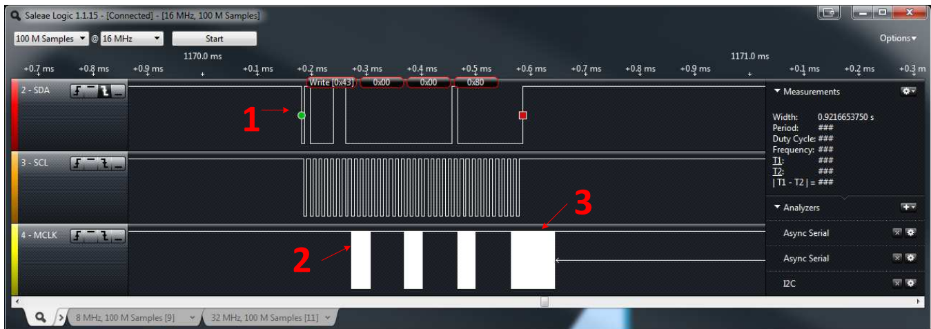
Figure 45. Power Profile for WriteWord Packet—Slave Using MSP430G2553
