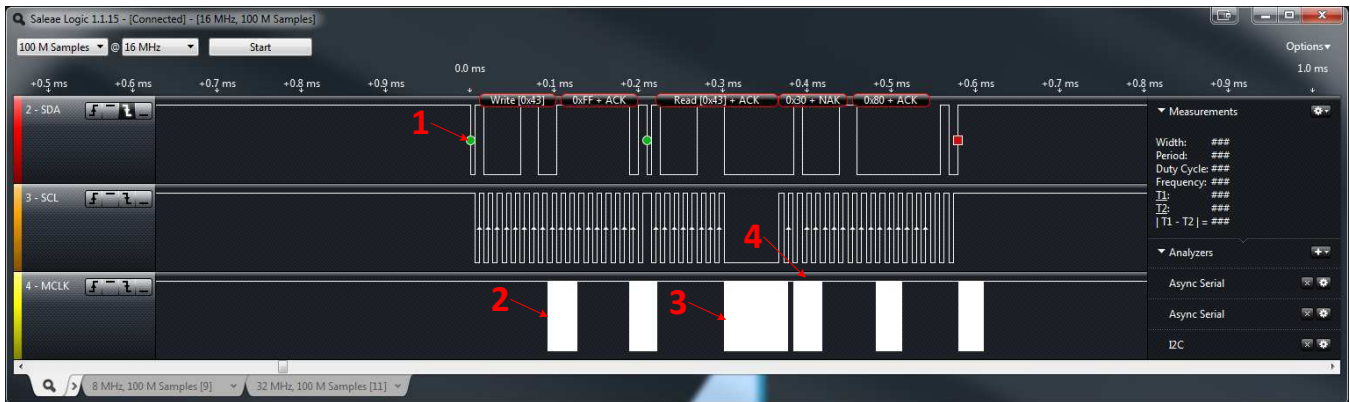
Figure 44. Power Profile for ReadWord Packet—Slave Using MSP430G2553
