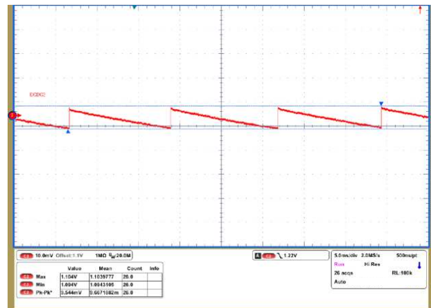
Figure 17. DCDC2 Output Voltage Ripple (Light Load, PFM)
