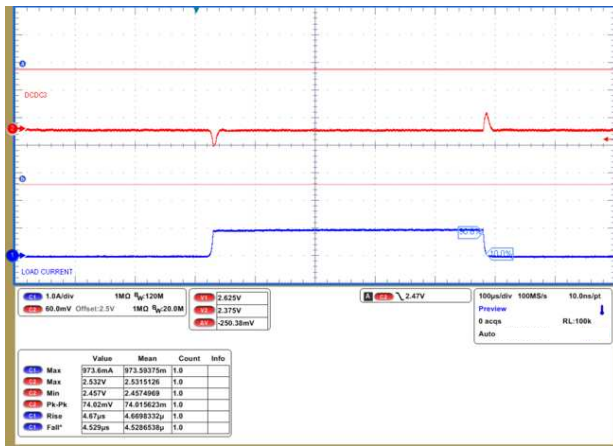
Figure 23. DCDC3 Load Transient Response (50 mA to 624 mA)
