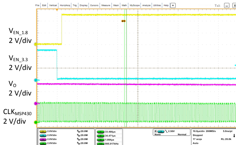
Figure 12 MSP430 Supply Changing from 3.3V to 1.8V
