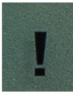
Figure 26. Symbol for Indicating Magnetic Tampering is Currently Detected
