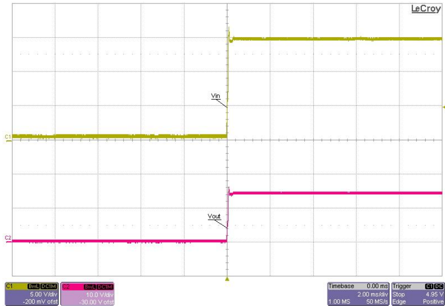
Figure 26: Startup into no load (current sense comparator reference voltage set to 2.4V) at 15Vin. Ch1 (yellow trace): Vin, Ch2 (pink trace): Vout
