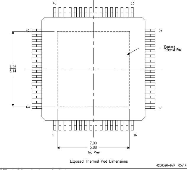
NOTES: A. All linear dimensions are in millimeters PowerPAD is a trademark of Texas Instruments
