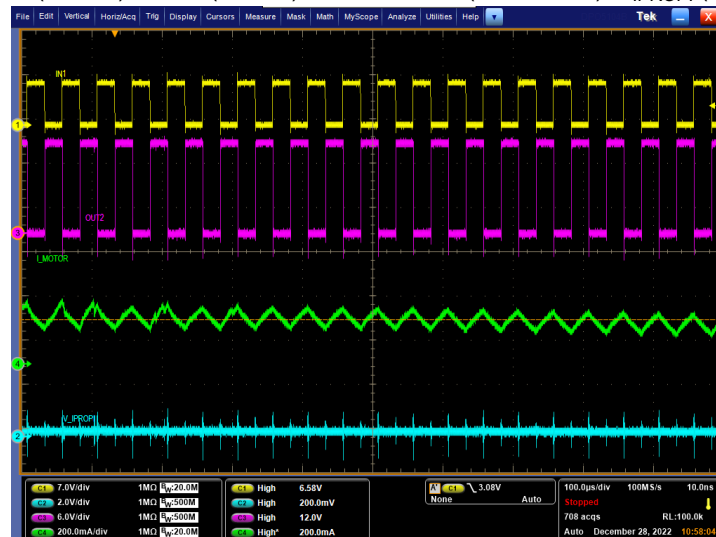
Figure 9-8. PWM Operation at VM = 11 V
