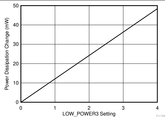
Figure 6-11. Power Dissipation Change vs LOW_POWER3 register setting
