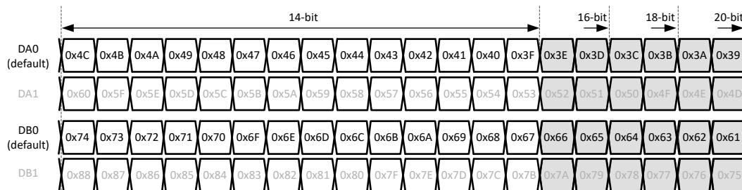
Figure 7-45. 1-wire output bit mapping
