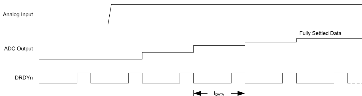
Figure 7-18. SINC3 Filter Behavior During Input Step Change
