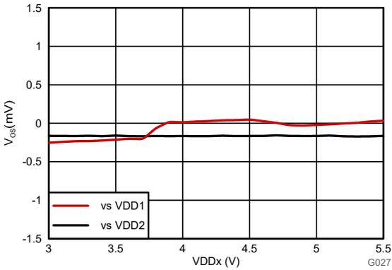
**Figure 6-6. Input Offset Voltage vs Supply Voltage**
