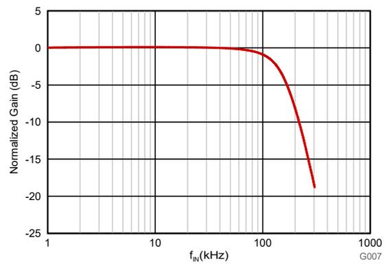
**Figure 6-11. Normalized Gain vs Input Frequency**
