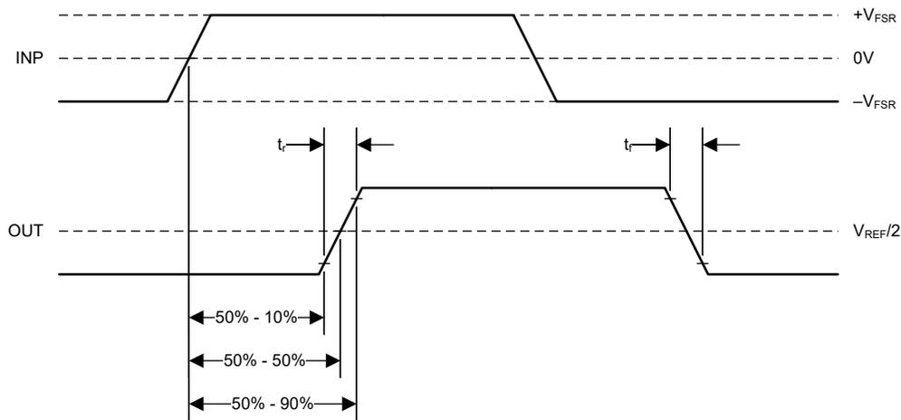
**Figure 6-1. Rise, Fall, and Delay Time Definition**
