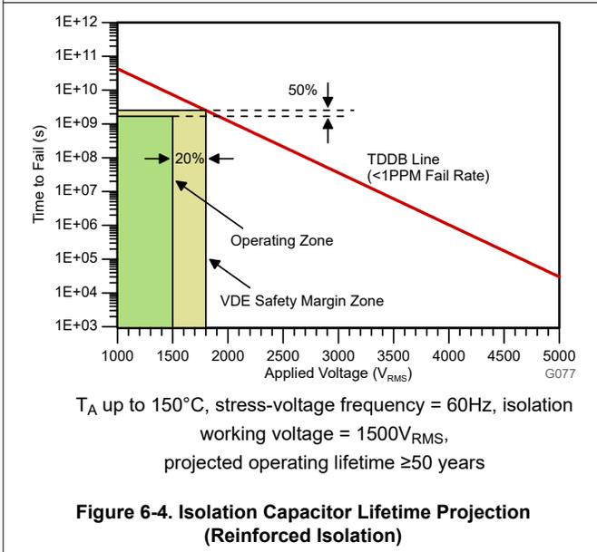
Figure 6-4. Isolation Capacitor Lifetime Projection (Reinforced Isolation)
