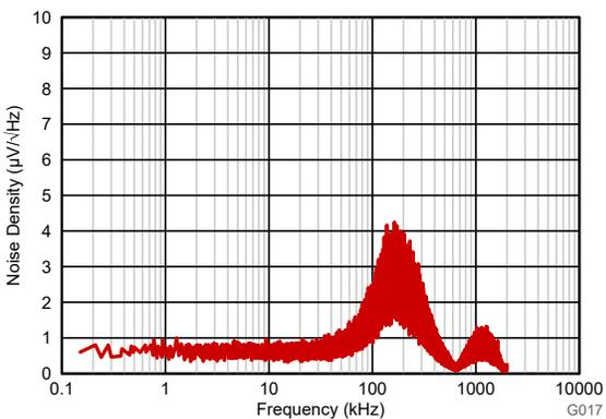
**Figure 6-10. Input-Referred Noise Density vs Frequency**
