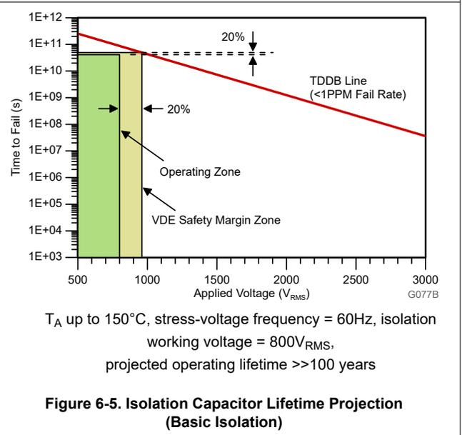
Figure 6-5. Isolation Capacitor Lifetime Projection (Basic Isolation)
