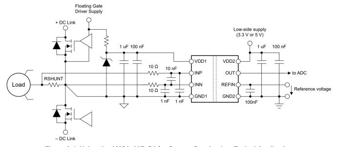
Figure 8-1. Using the AMC0x02R-Q1 for Current Sensing in a Typical Application
