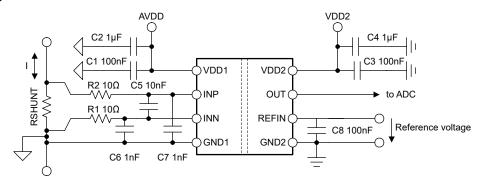
Figure 8-6. Decoupling of the AMC0x02R-Q1
