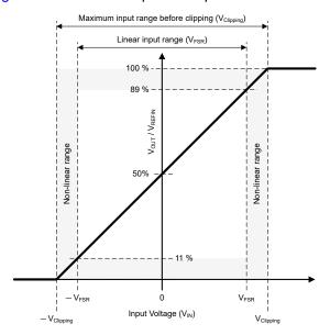
Figure 7-3. Input-to-Output Transfer Curve of the AMC0x02R-Q1
