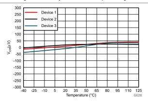
Figure 6-9. Input Offset Voltage vs Temperature
