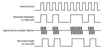
Figure 7-2. OOK-Based Modulation Scheme
