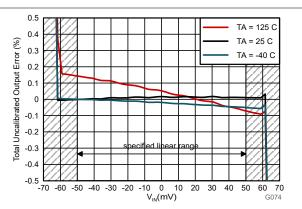
Total uncalibrated output error is defined as:((V<sub>OUT Measured</sub> - V<sub>OUT Expected</sub>) / V<sub>REFIN</sub>) x 100 , where V<sub>OUT Expected</sub> = V<sub>IN</sub> /  $V_{Clipping} \times V_{REFIN} / 2 + V_{REFIN} / 2$ ,  $V_{REFIN} = 3.3V$  and  $V_{Clipping} =$
