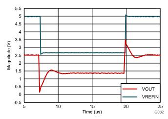
Figure 8-5. Reference Input Step Response of the AMC0x02R-Q1
