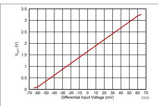
Figure 6-6. Output Voltage vs Input Voltage
