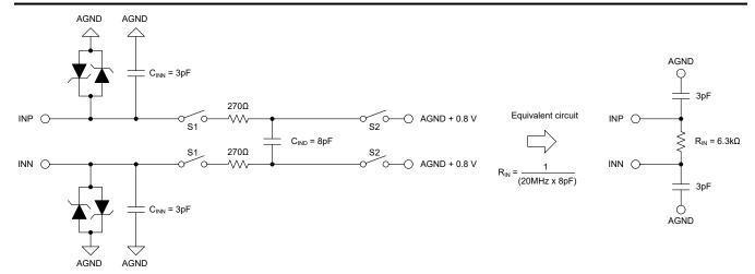
Figure 7-1. Equivalent Input Circuit
