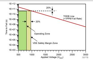
T<sub>A</sub> up to 150°C, stress-voltage frequency = 60Hz, isolation working voltage = 800V<sub>RMS</sub>, projected operating lifetime >>100 years
