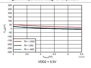
Figure 6-11. Input Offset Voltage vs VREFIN
