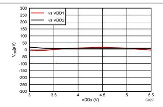
Figure 6-8. Input Offset Voltage vs Supply Voltage
