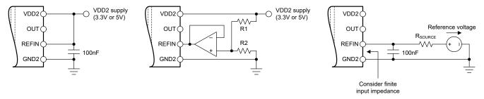
Figure 8-3. Connecting the REFIN Pin
