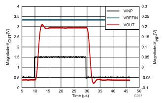
Figure 8-4. Output Step Response of the AMC0x02R-Q1
