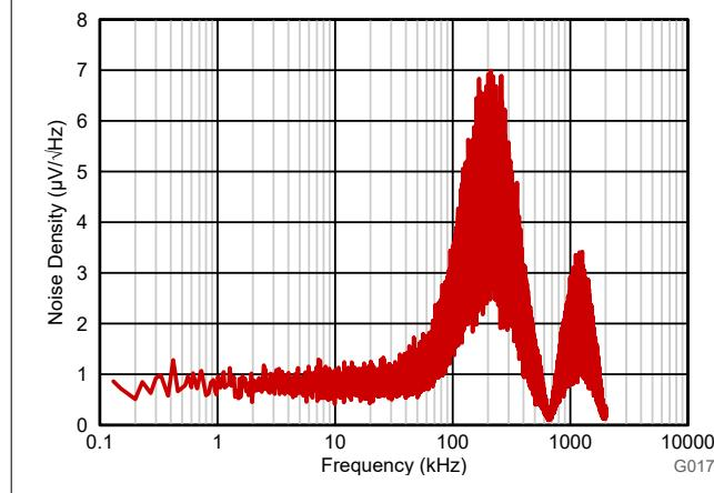
Figure 6-10. Input-Referred Noise Density vs Frequency
