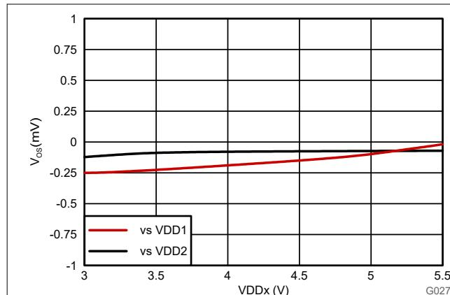
Figure 6-6. Input Offset Voltage vs Supply Voltage
