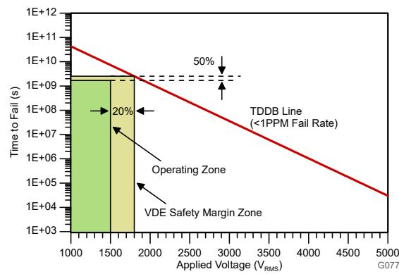
$T_A$  up to 150°C, stress-voltage frequency = 60Hz, isolation working voltage = 1500V<sub>RMS</sub>, projected operating lifetime  $\geq$  50 years
