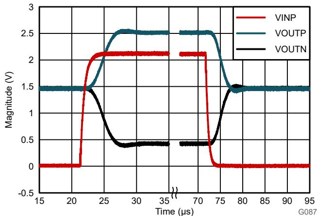
**Figure 8-4. Step Response of the AMC0x11D-Q1**
