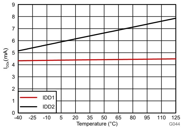
Figure 6-14. Supply Current vs Temperature
