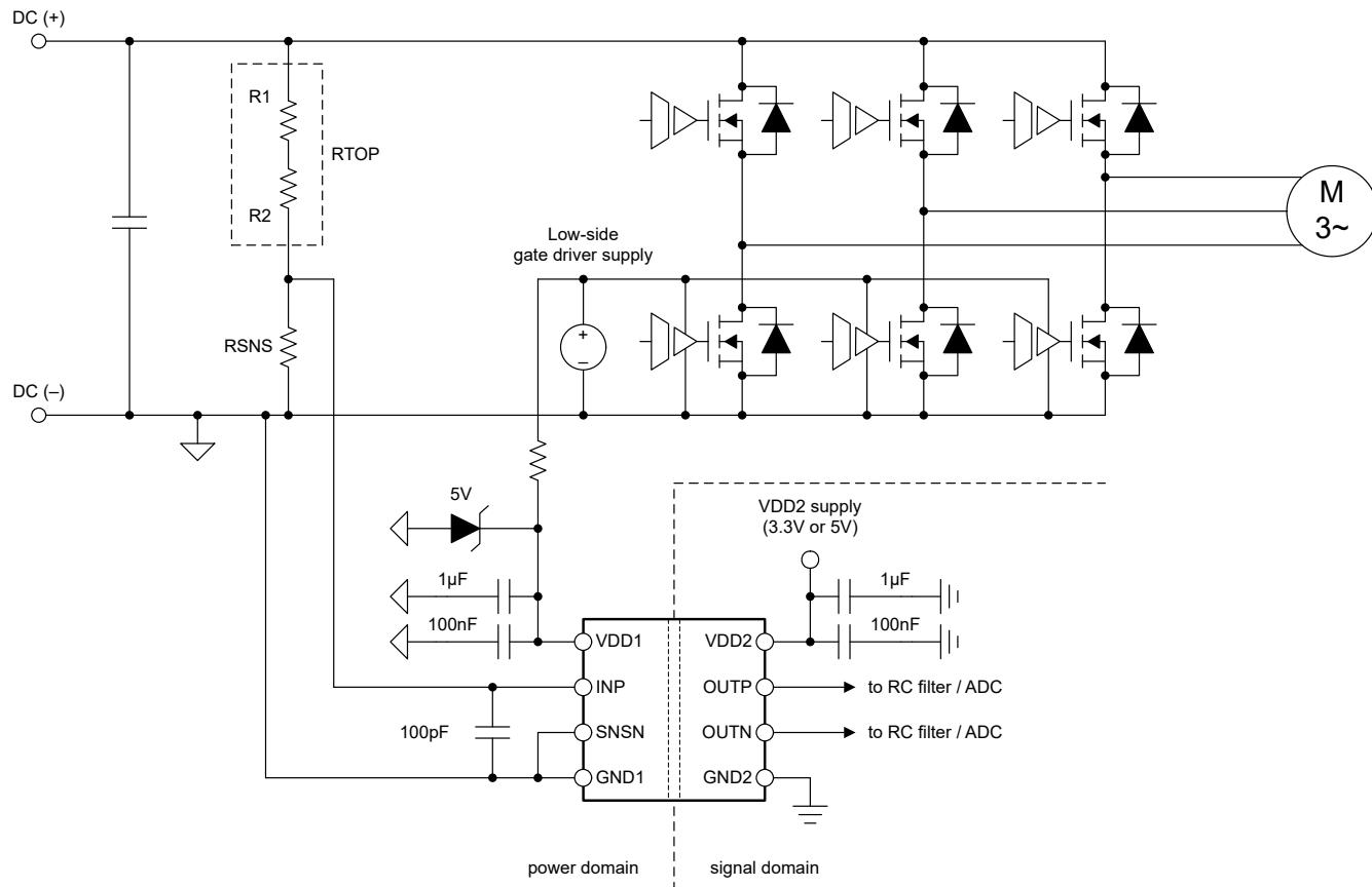
Figure 8-1. Using the AMC0x11D-Q1 in a Typical Application
