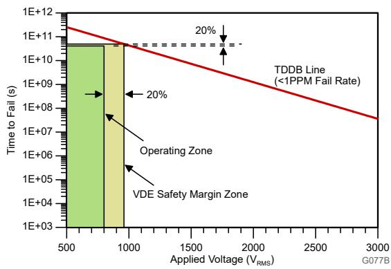
$T_A$  up to 150°C, stress-voltage frequency = 60Hz, isolation working voltage = 800V<sub>RMS</sub>, projected operating lifetime  $>> 100$  years
