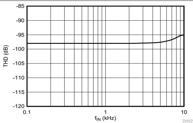
**Figure 6-27. Total Harmonic Distortion vs Input Signal Frequency**
