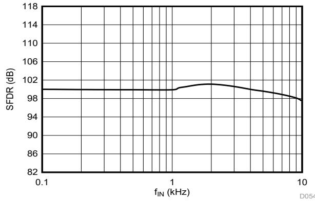
Figure 6-32. Spurious-Free Dynamic Range vs Input Signal Frequency
