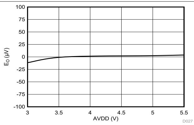
Figure 6-11. Offset Error vs High-Side Supply Voltage
