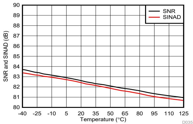
Figure 6-19. Signal-to-Noise Ratio and Signal-to-Noise + Distortion vs Temperature
