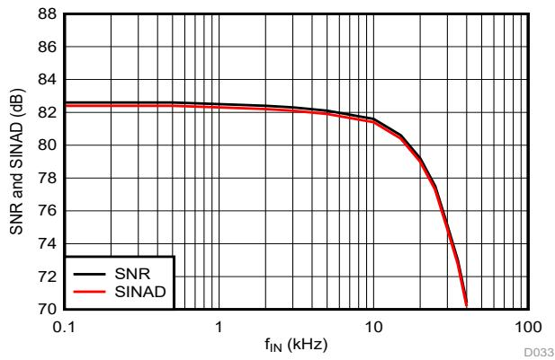
Figure 6-21. Signal-to-Noise Ratio and Signal-to-Noise + Distortion vs Input Signal Frequency
