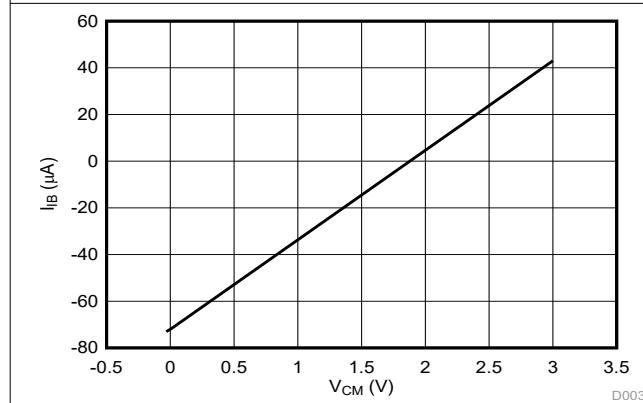
Figure 6-8. Input Bias Current vs Common-Mode Input Voltage
