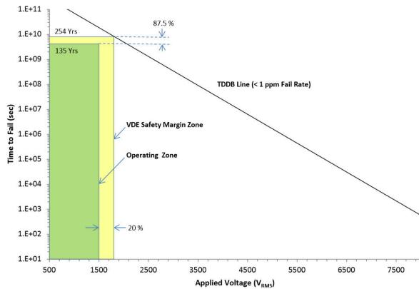
TA up to 150°C, stress-voltage frequency = 60 Hz, isolation working voltage = 1500 V<sub>RMS</sub>, operating lifetime = 135 years
