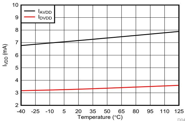
Figure 6-37. Supply Current vs Temperature
