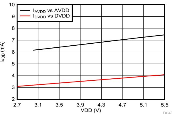
Figure 6-36. Supply Current vs Supply Voltage
