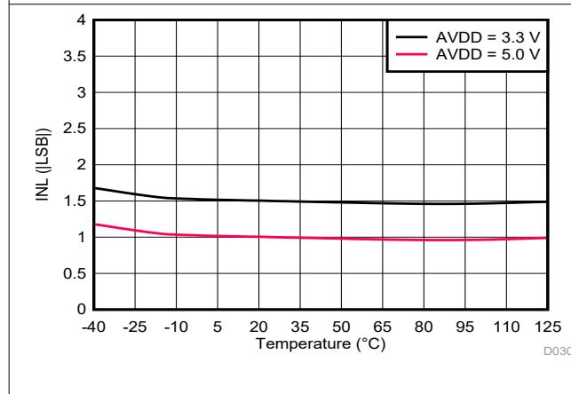
Figure 6-10. Integral Nonlinearity vs Temperature
