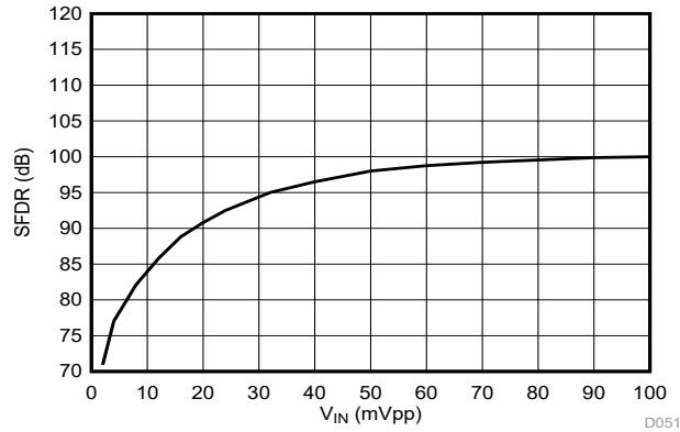
Figure 6-33. Spurious-Free Dynamic Range vs Input Signal Amplitude
