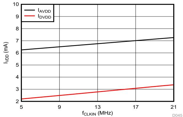
Figure 6-38. Supply Current vs Clock Frequency
