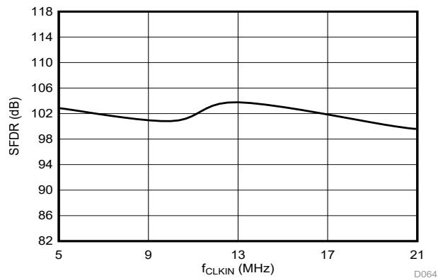
Figure 6-31. Spurious-Free Dynamic Range vs Clock Frequency
