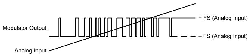
**Figure 7-4. AMC1306M05-Q1 Modulator Output vs Analog Input**
