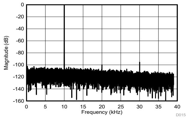
Figure 6-35. Frequency Spectrum With 10-kHz Input Signal
