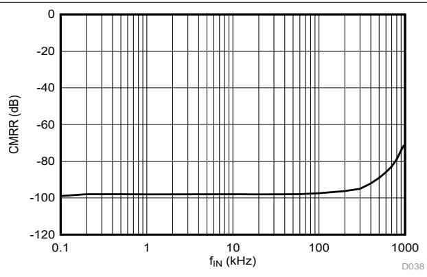
Figure 6-9. Common-Mode Rejection Ratio vs Input Signal Frequency
