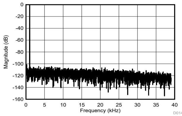
Figure 6-34. Frequency Spectrum With 1-kHz Input Signal
