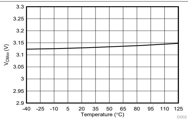
Figure 6-7. Common-Mode Overvoltage Detection Level vs Temperature
