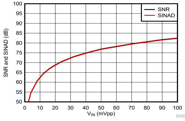
Figure 6-22. Signal-to-Noise Ratio and Signal-to-Noise + Distortion vs Input Signal Amplitude
