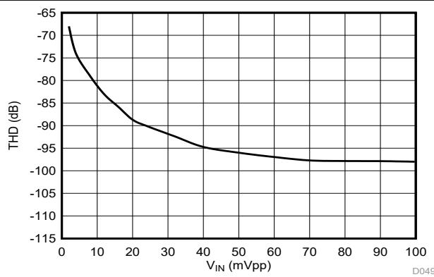
**Figure 6-28. Total Harmonic Distortion vs Input Signal Amplitude**
