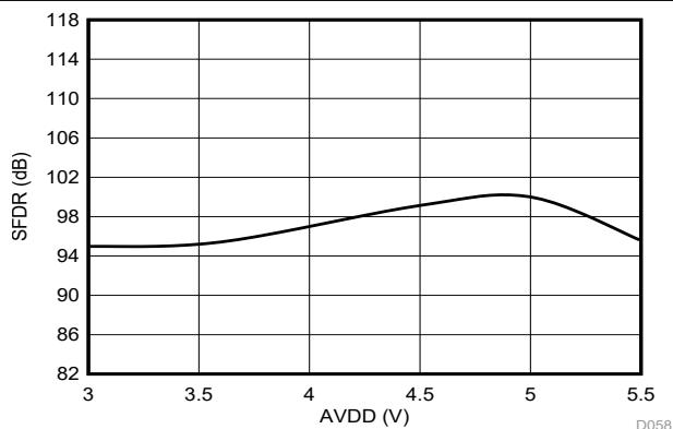
**Figure 6-29. Spurious-Free Dynamic Range vs High-Side Supply Voltage**
