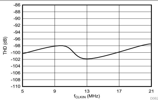
**Figure 6-26. Total Harmonic Distortion vs Clock Frequency**
