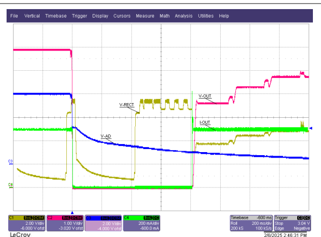
Figure 9-6. Transition Between Wired Power and Wireless Power (EN1 = EN2 = LOW)
