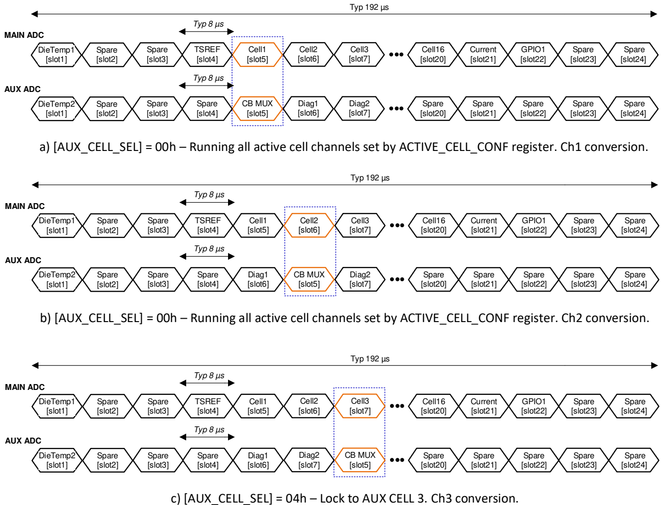
Figure 9-11. Synchronization between MAIN and AUX ADC Sampling
